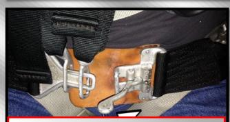
6. Lift up to remove shoulder harness and seat belt (No need to remove parachute , pilot can be lifted up with parachute attached
