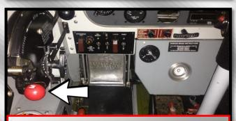
3. Squeeze metal tab and pull the red fuel mixture control nob aft this shuts off engine
