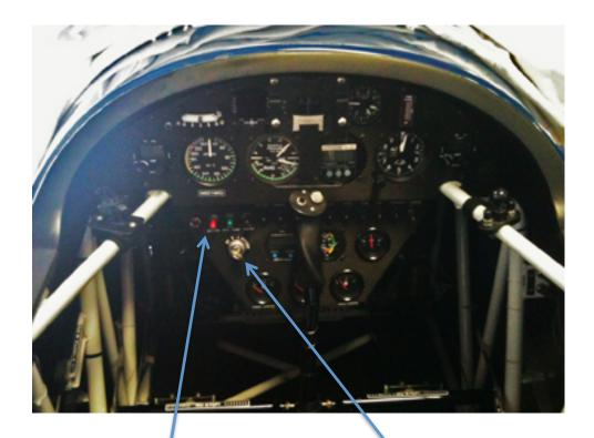
The master switch, controlling all avionics and battery is a small red lever located on the left/bottom portion of the instrument panel. Flip the switch down to turn off.
