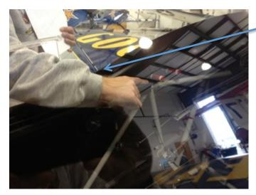
Insert right arm into cockpit through window.
