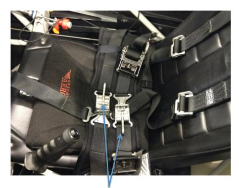
To release belt, locate the two silver levers at the center of the belts. Lift the rounded end of each lever away from the torso.
