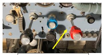
Mixture: push on center button and pull back until it stops
