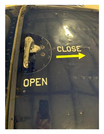
Turn latch (on top of canopy) to OPEN position, slide canopy aft
