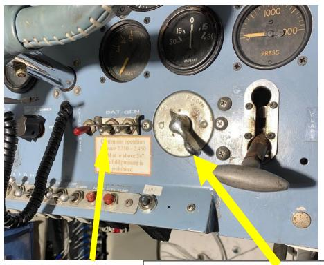
Battery / Alternator switches \_ push these down for OFF
