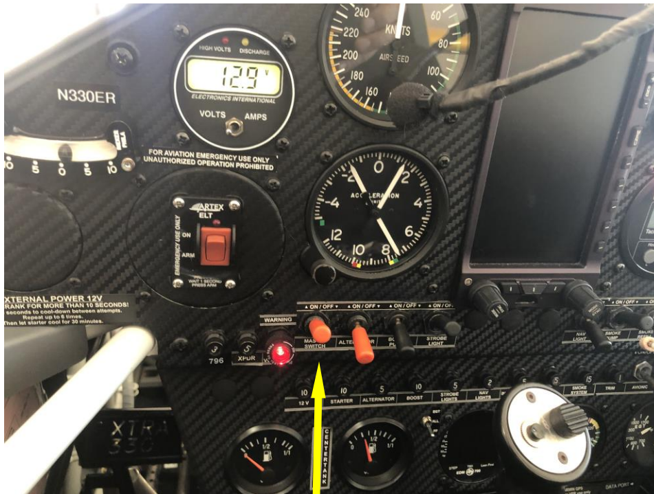
Master Power Switch– DOWN IS OFF
