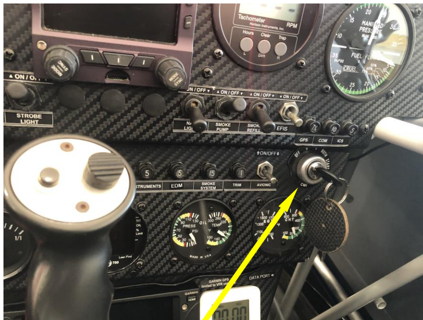
Ignition / Starter Switch– Full CCW is OFF
