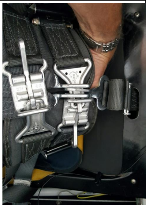
Both lap belts latched Lower latch: Shoulders, Laps and Crotch Upper latch: Redundant Lap
