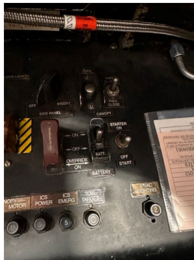
BATTERY SWITCH (FRONT AND REAR THE SAME)
